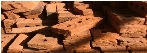
Fig 6.1 Improper way of storing
